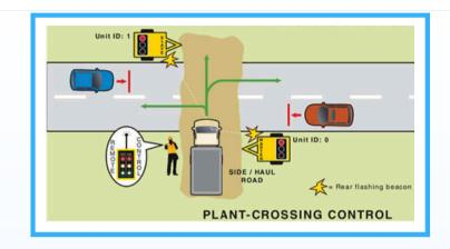
These **TTS units** can work in conjunction with **Trailer Traffic Lights** and can be set to do up to an **8-way configuration**.
